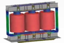
Pennsylvania Transformer Technology, Inc. performed multiphysics simulations using Maxwell, ANSYS Mechanical and ANSYS CFD to design next-generation transformers for the utility power industry.
